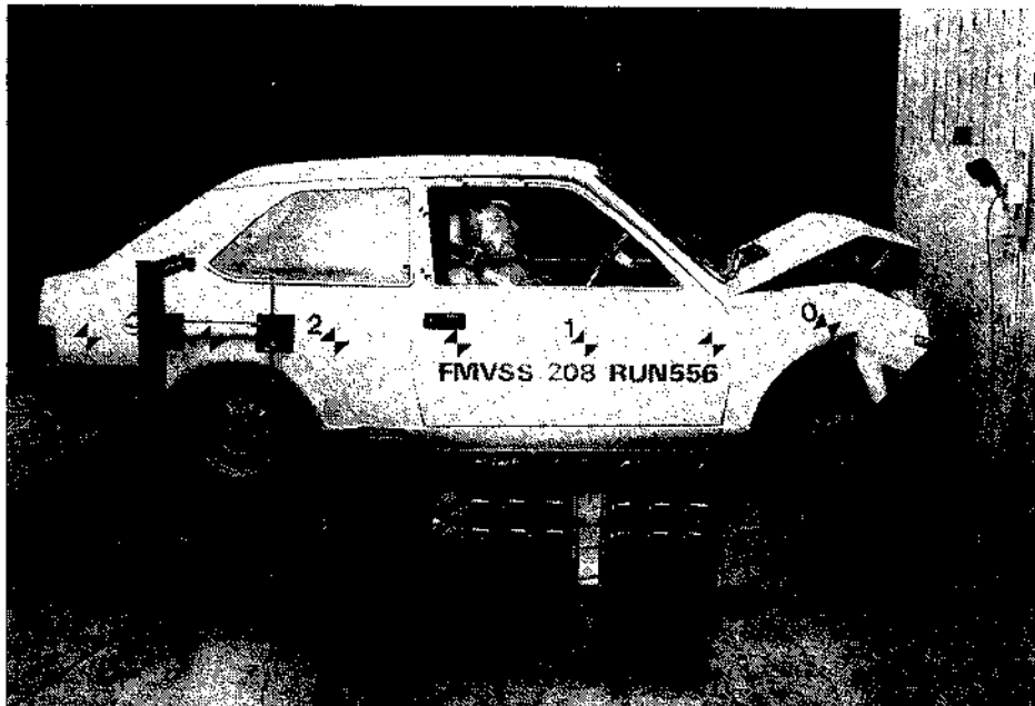
Fig. 7.17 A head-on collision of a passenger car against a fixed barrier (concrete block) in accordance with a US standard.
