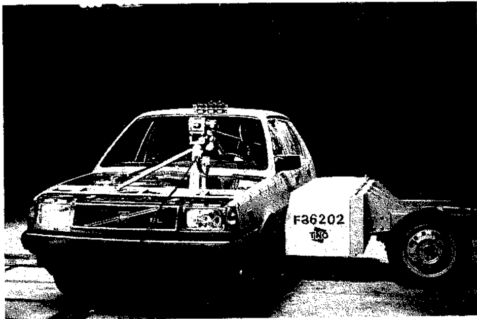
Fig. 7.27 Side impact of a moving deformable barrier against a passenger car.
